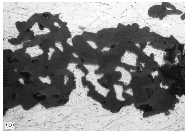
Figure 12 (a, b) Cross-sections of specimens pre-treated in argon plus annealed in oxygen.
